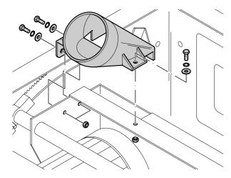
If you are using a dust collector, connect to the chip case's suction port.
